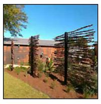
**Feature wall on the garage** was painted with Porter's Rusting Paint. This was applied with two coats; the first coat contains metal particles, the second coat was a wash containing a rusting agent (HCI) which gives the patina.
